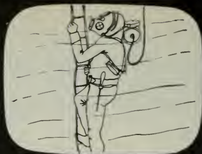
1872 FACE MASK and compressed air apparatus by Rouquayrol-Denayrouze introduced the equalized air pressure.
